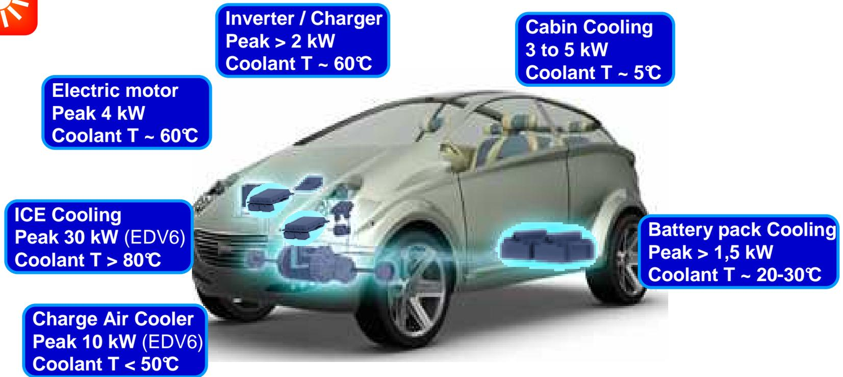
BTM integration into the overall thermal architecture
